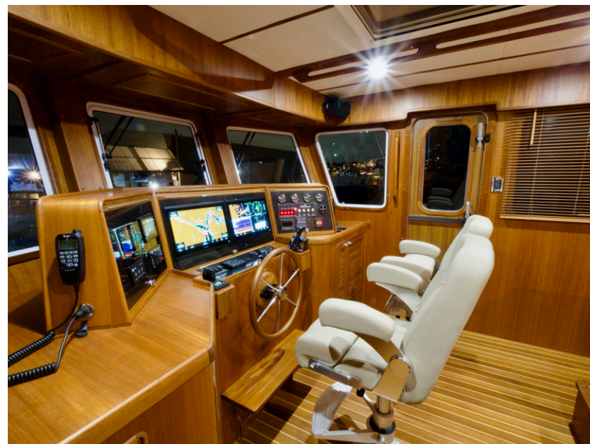
Above: The U-shape galley is open to the salon and includes plenty of refrigerator and freezer capacity, stowage and countertop space. Below: Redundant systems in the wheelhouse include two chartplotters, three VHF radios, Starlink and AIS.
